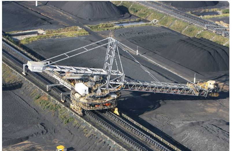
Existing SR3 Stacker/Reclaimer that will be significantly upgraded and repositioned on Bund 6
